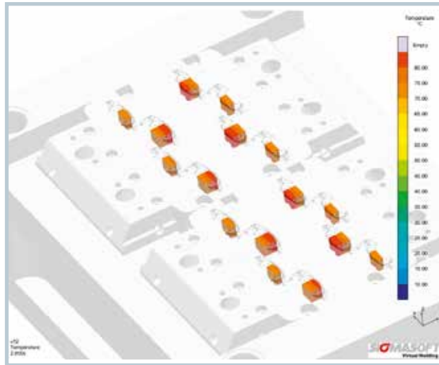
Fig. 3. Hotspots form in the slide cores with temperatures over 70°C (© Sigma Engineering)
